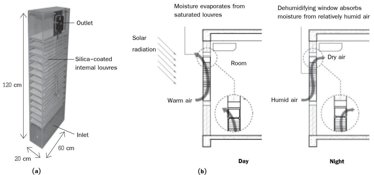
**Figure 13.** Dehumidifying window (a) and its operation (b) [111].
