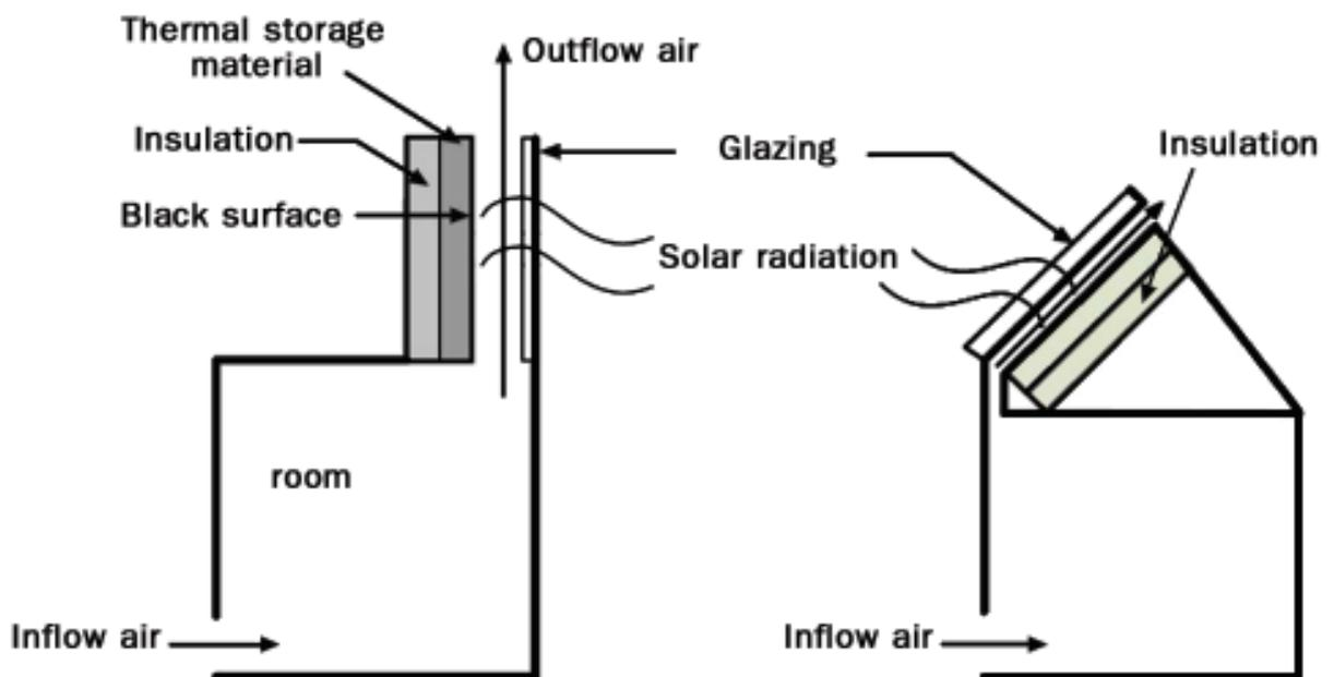
**Figure 7.** Examples of solar chimney configurations: vertical (a) and inclined (b) (adapted from [90]).
