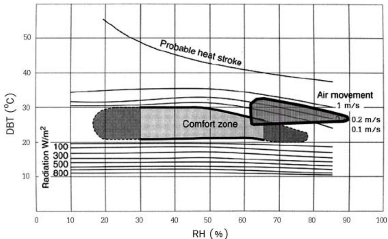
**Figure 1.** Bioclimatic chart modified for hot humid climates (adapted from Olgyay [31] following Jitkhajornwanich [15]). The new comfort zone is shown on the right of the original one.
