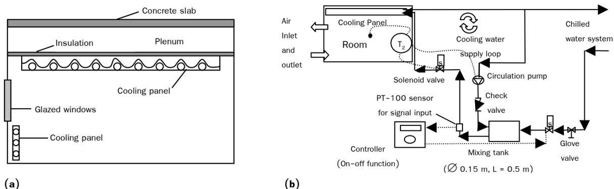
**Figure 10.** A schematic of the cool radiant panel system tested in Thailand (adapted from [103]). Figure 10a shows a section indicating the location of the radiant panels in the test room. Figure 10b shows the diagram of the cool-water circulation system.
