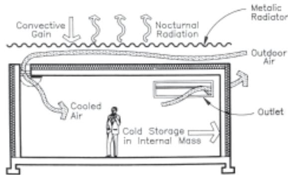
**Figure 9.** A schematic of a radiant cooling system which involves cooling the roof by nocturnal radiation and introducing cooled night air into the occupied space [5].
