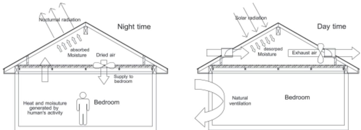
**Figure 12.** A schematic of the dehumidification system that uses an attic as a dehumidification chamber (adapted from [110]).
