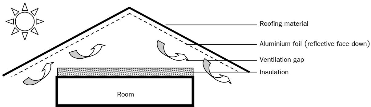
**Figure 4.** A schematic of a roof section showing an example of a combined use of insulation, a ventilation space and reflective lining to minimise thermal impact from solar radiation on the interior environment.
