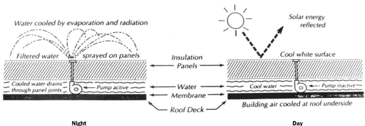
Figure 11. A schematic of the Coolroof system (i.e. roof pond with floating insulation; adapted from [5]).
