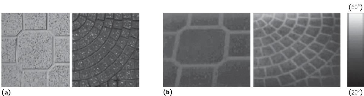
**Figure 5.** Visible (a) and infrared (b) images of light and dark paving materials under direct sun [62]. Darker colours in the infrared image represent lower temperatures. The temperature scale is given on the right.
