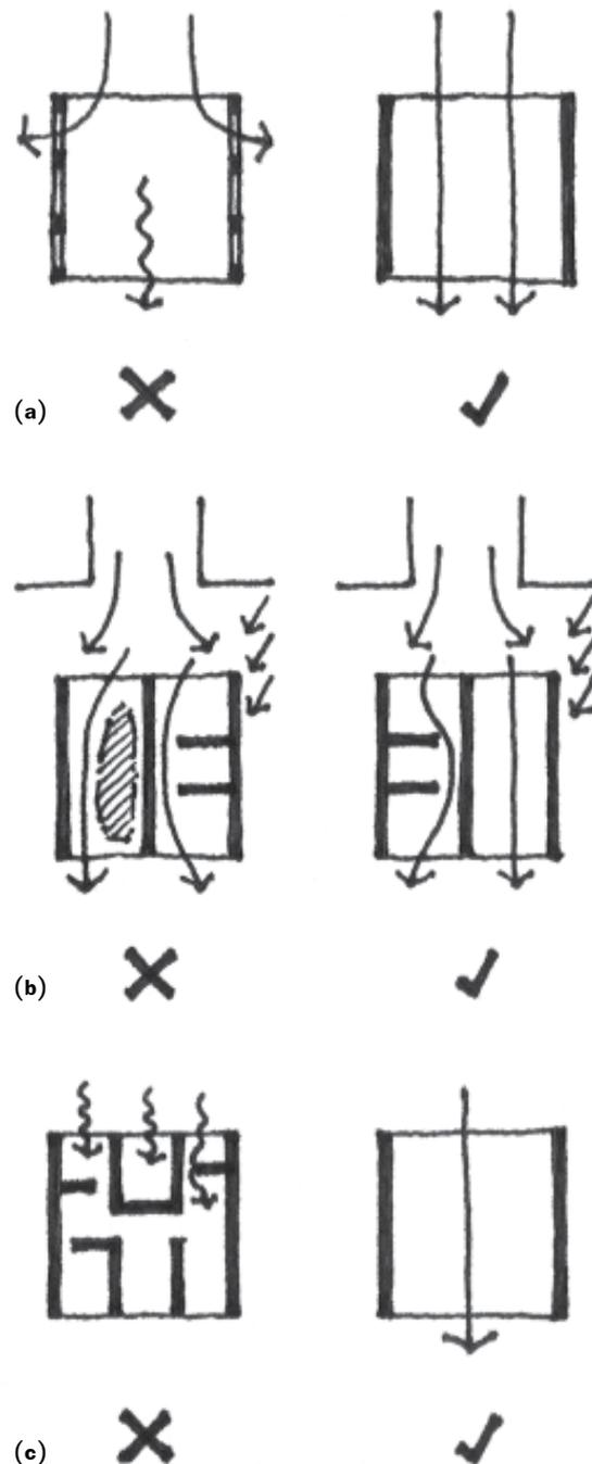
**Figure 6.** Examples of opening design to encourage interior air movement [36].
