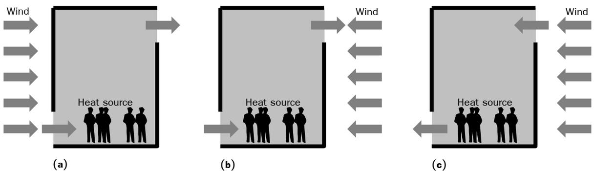
**Figure 8.** Wind-assisted ventilation (a); buoyancy dominated, wind-opposed ventilation (b); and wind dominated, wind-opposed ventilation (c).
